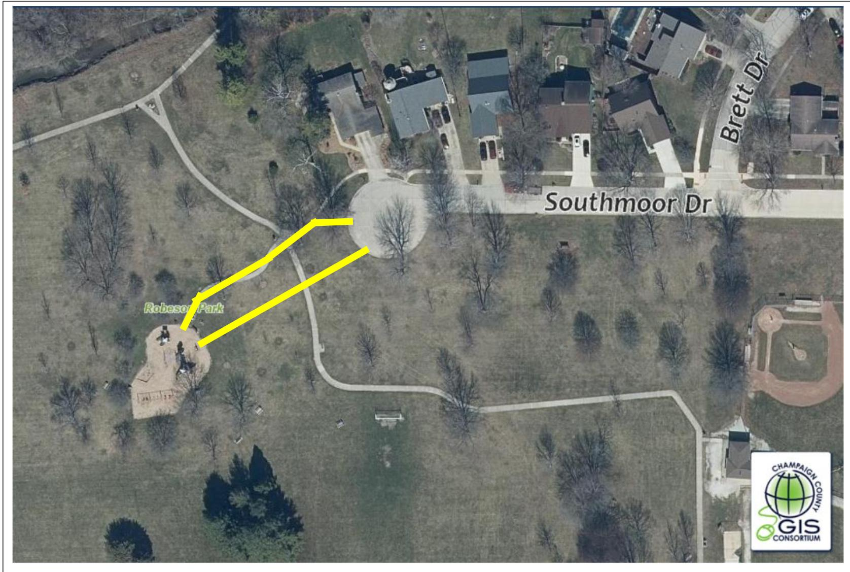
**Exhibit B** - Robeson Park sidewalk to playground in which existing condition (slope) does not meet ADA requirements is shaded in yellow. Approximate location of placement of under-sidewalk drainage by white line. Exact slopes and measurements to be determined by bidder.
